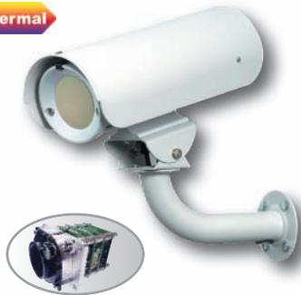
A compact thermal imaging camera offering high contrast, real-time thermal video at an affordable price. Using a microbolometer detector with a germanium lens, the video image is displayed from an interpolated heat signature emitted from people, vehicles, structures, electrical and mechanical components, etc. Ideal applications include perimeter surveillance, search and rescue, marine and port security, border patrol, electrical inspection, moisture detection and energy conservation.
