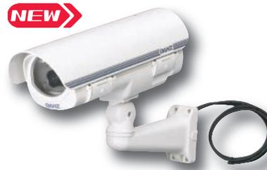
This environmental housing kit is designed to accommodate most camera & lens combinations including 10X varifocals and 6X motorized zoom lenses. The kit includes a 24VAC heater, sunshield, and pre-wired power and video cable for quick and easy installation in the field.
