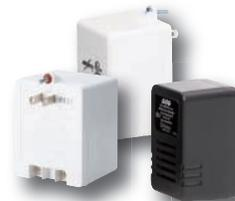
Three models offer solutions to meet different installation requirements. The C12DCR-500 provides 12 volts DC regulated 500 milliamps output; the C24AC provides 24 volts AC 20vA output; and the C24AC-40 provides 24 volts AC 40vA. The power supplies are UL-listed and plug into any 120 VAC duplex wall receptacle. For indoor use only.
