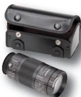
A valuable tool for both the seasoned professional and first-time installer. The viewfinder is an optical tool to help determine the required focal length. First look through the eyepiece and zoom in to the desired image. Then read the required focal length on the lens barrel. Covers 2/3", 1/2", 1/3", and 1/4" formats. A protective case and neck strap are included.
